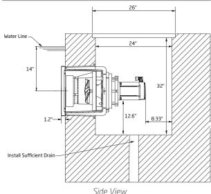
NOTE: Patented combined suction and discharge fitting does not require main drains.
